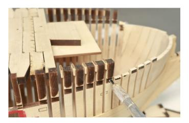
With the extensions removed for all of the cant frames we are almost done. Now we must tackle the jigs for the square frames. I am just using the very same scroll saw blade to cut the top timber extension on the port side. Then I do the same to the top timber extension on the starboard side and the cross jig for that square frame will be freed.
