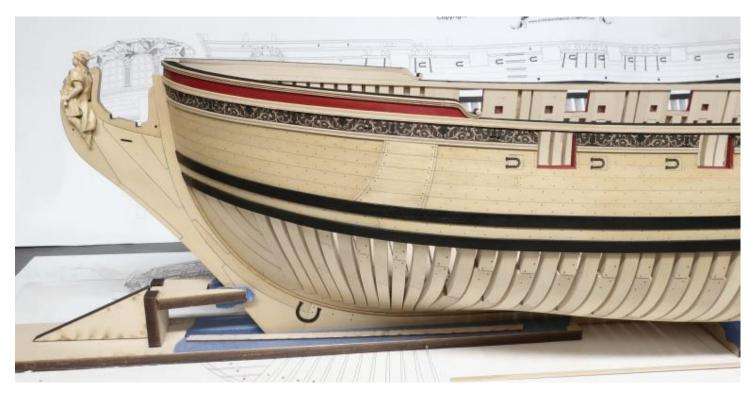
the scroll so the pattern of laser etched detail matched as close as possible. Repeat the same process at the bow. See the photos provided.
