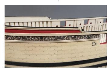
require some tweaking. Then position and glue the molding strip in position. But it up against
