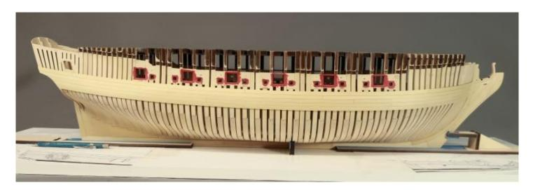
Remember that the strakes for the wales have no taper at the bow. Those are straight 7/32" wide strips. BUT, the next five strakes above the wales do taper at the bow as discussed. Yes it's weird but that is how it was done on the contemporary model. I am just following suit for our model as well.
