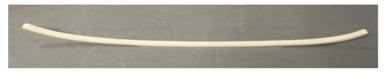
120 grit. Remember when you are doing this NOT to reduce the fairing cap. Its inevitable that you may hit it from time to time and you may remove the laser char but try and keep the width of the sheer as consistent as you can. The fairing cap helps you do this. Here is a picture after finishing up the inboard fairing. Now I can return to the outboard
