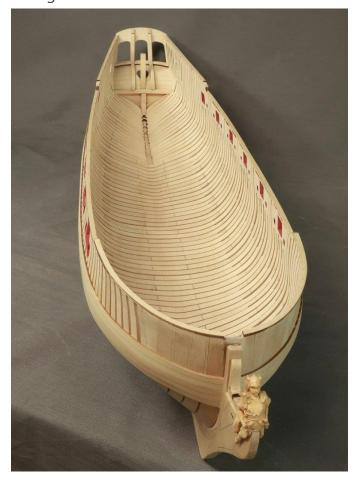
planking with a much cleaner hull. Although I am compelled to add the keelson first just to make the inboard area even cleaner, it's nice NOT to have to look at all that unkempt framing and laser char. It cleaned up rather well dont you think?
