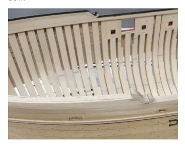
With the scroll cap glued in position, you can sand the inboard and outboard sides flush with the planking. You can also fill any gaps along the planking and the scroll cap but this will ultimately be painted and covered up anyway.
