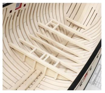
Planking is underway with 5/16" x 3/64" cedar strips. I am not too concerned about getting up close to the sides of the hull. Depending on how fairing went, this could sometimes lead to a weird shape along the edge of the platform.
