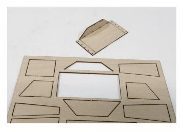
8. Add the two sides. You will need to bevel the bottom to sit flush on the base.
