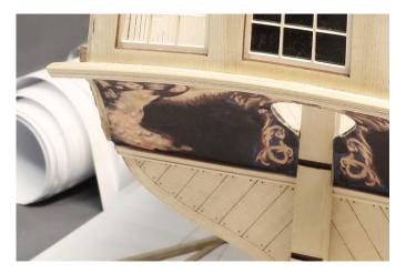
Then the sides are completed and trimmed. But before you can do that, cut a small length of 1/8" x 3/32" strip (use scrap) and glue it onto the side of the hull. See it below just under the serpent's snout.
