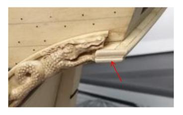
To complete this step...another small length of scraped molding is glued on top to finish it off. This creates a nice sized platform where the side figures will sit. You can shape to suit your own sensibilities and have the standing figure with you to test as you finalize this ledge. Its unclear on the contemporary model just how this is shaped but this was a good reconstruction. I filled any cracks with wood filler in preparation for the transom carvings next.
