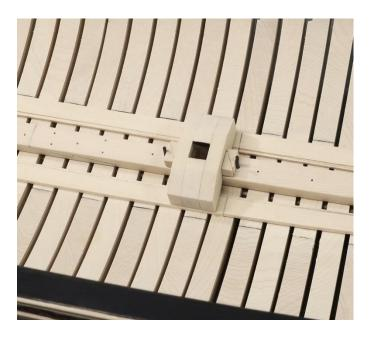
With the limber strakes completed, the mast steps can be assembled and installed. I would also note that I didn't bother treenailing the limber strakes because it will just not be seen. But you can do that if you feel compelled.
