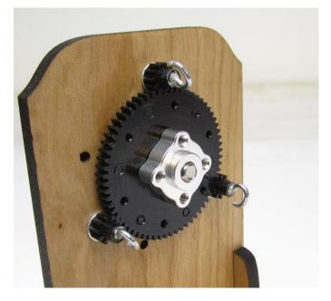
To finish it up, insert the four set screws into the face of the shaft hub and secure them with loc-tite. You won't
