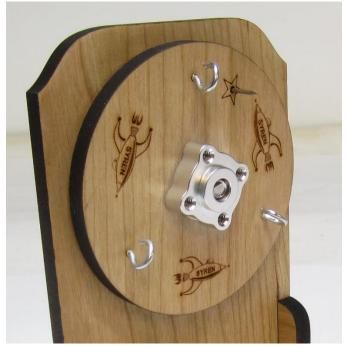
Then afterwards tighten the set screw on the side of the shaft hub to secure it to the machine screw. BUT make sure the disc turns freely after you tighten this set screw. It shouldn't be too tight with any friction afterwards. It should also not be too loose that it wobbles. Just tight enough so that it turns freely.
