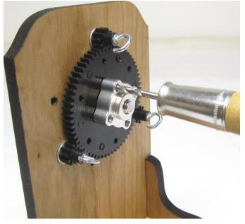
Tighten the set screw slightly to secure it for drilling.
