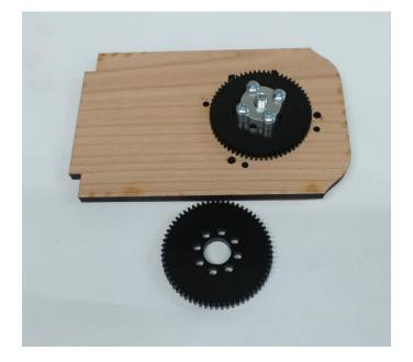
You can flip the hub around to secure it in the bore hole of the new style gear as it is a perfect fit. You
