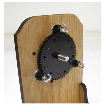
It should slip onto the machine screw easy enough with the plastic center shaft of the gear sliding into the center hole of the upright.
