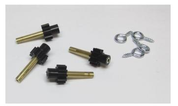
Take the four small gears and the four short lengths of brass tubing. Insert the brass tubes into the bore of the gears. You can use a small hammer to gently drive the tubes into the bore. It will be a very tight fit as it should be and it will be impossible to remove them. So study the photo above carefully so you orient the gears properly on the tube ends. Make sure they face the right way!!!
