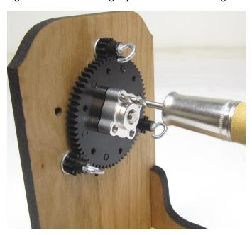
Then drill those four 3/32" holes through the gear. Enlarge them slightly so the four small set screws will fit snug into them. Clean up any plastic burrs on the gears with some sandpaper and place it back onto the machine screw.
