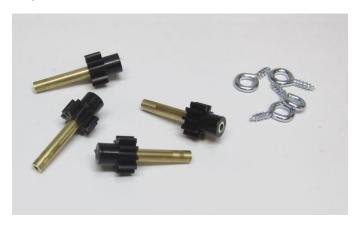
Take the four small gears and the four short lengths of brass tubing. Insert the brass tubes into the bore of the gears. You can use a small hammer to gently drive the tubes into the bore. It will be a very tight fit as it should be and it will be impossible to remove them. So study the photo above carefully so you orient the gears properly on the tube ends. Make sure they face the right way!!!
