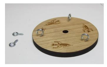
To complete step one, take the two laser cut discs and insert the screw eyes into the laser cut pilot holes.
