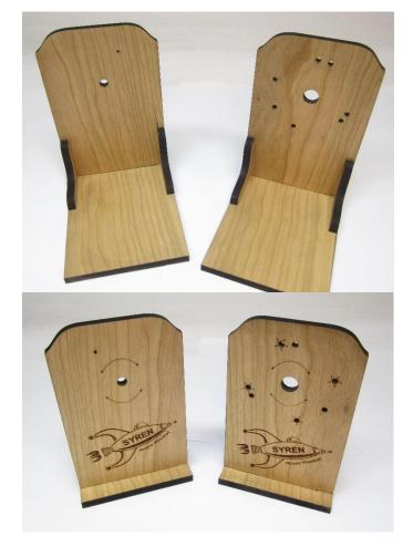
Sand the surfaces well and apply several coats of wipe on poly or other protective finish.
