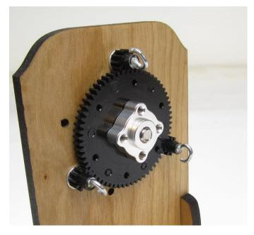
To finish it up, insert the four set screws into the face of the shaft hub and secure them with loc-tite. You won't be removing this large gear again so make sure it is secure. After you tighten the set screw on the side of the shaft hub, make sure the gears will turn freely. Remember to tighten this set screw well and crush those threads on the machine screw to create a flat.
