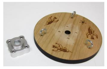
Then loosen and remove the shaft hub so you can enlarge the holes in the wood disc slightly. You can use a needle file or even a larger 7/64" drill bit. The four holes don't even need to go all the way through the disc. These holes are just to register the disc against the shaft hub with set screws in the next step. You can repeat this process with the 4-strand disc also but in step four, set up the tail stock with the 3-strand disc in preparations for your rope making tutorials.
