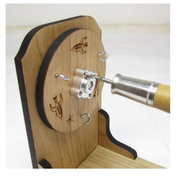
Tighten the set screw on the side of the shaft hub to fully secure the shaft hub against the wood disc.
