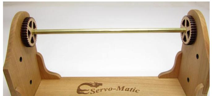
**Step 7** – Insert the two smaller shafts into the two remaining gears as shown. Yes, there are two different sizes of shaft if you were wondering. Try to ensure that the gears are not crooked...nobody like a wobbly gear. These should be glued to the tubes but make sure the tube is slid all of the way
