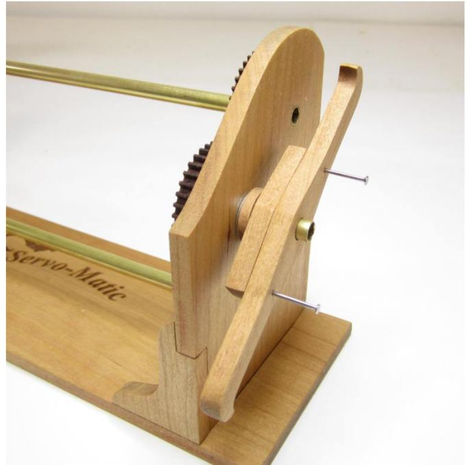
**Step 11 – Repeat this process on the other side with the diamond piece.** Slide the washer on first and then the wooden spacer washer followed by the diamond shaped piece. Glue it into position.
