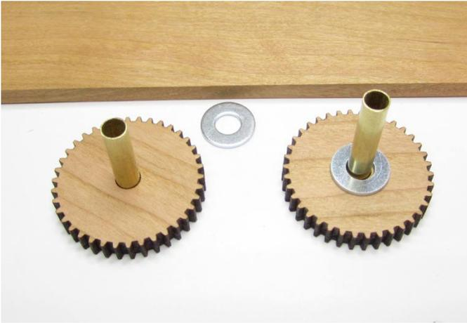
through the gears. Do this on the table top as shown in the photo. Place two metal washers on the shafts. Also be sure to file the edges of these tubes to debur them. Give them a dull edge so they won't shred and cut the rope as you serve it. You can even add a drop or two of CA glue to the edges in order to dull them and smooth them out. Run the drop all around the edge of the tube opening.
