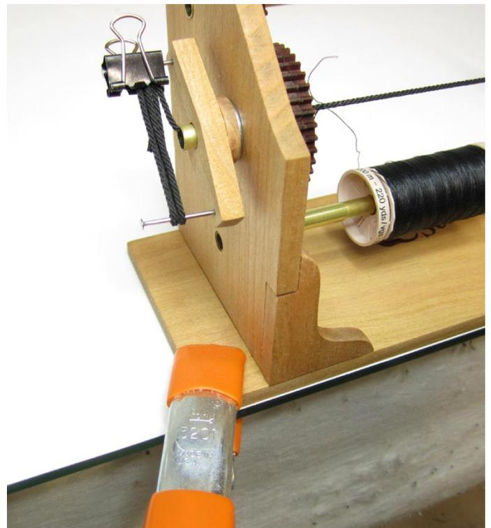
**It's also best to secure the machine to your work table using a clamp as shown. It will prevent the machine from moving and sliding as you serve the rope.**
