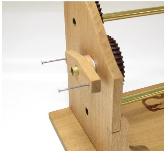
You are basically done building the machine. The left over long brass tube is slid through the remaining holes...**NO GLUE HERE** - this is the tube you will slide a bobbin of serving thread onto. You will need to be able to remove this so you can replace the bobbin as needed.
