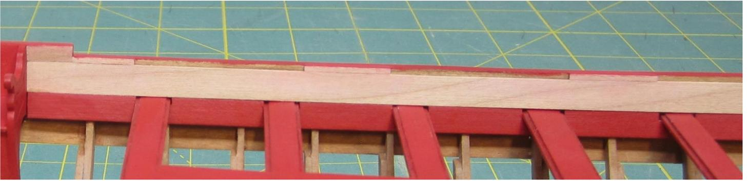
have to use the laser cut plank as a starting template only and cut a new plank from a 1/32" sheet of cherry so it is the correct width. Use it as a pattern to cut a wider version.
