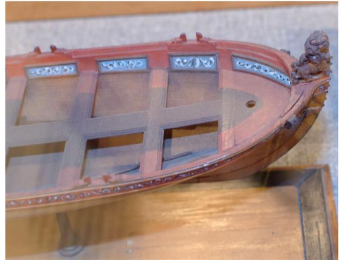
how it creates a decorative pattern along the edge of the cap rail inboard. The photo above shows this detail on a contemporary model of a barge. Examine the plans carefully for where these short lengths should be added because they alternate from one side of the barge to the other. The bottom photo shows these elements in position on our model. This is why it is so important that the initial plank only extend up to the bottom edge of the cap rail. If you placed your riser too low you may
