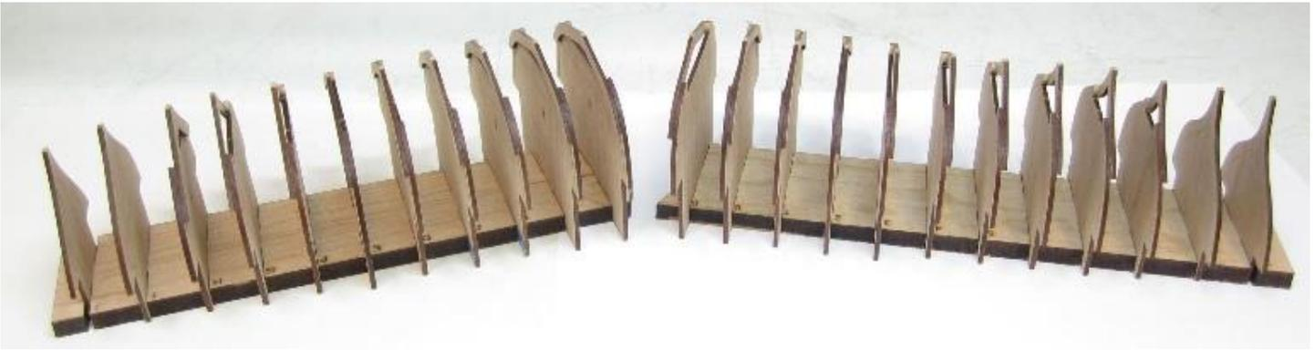
Remove all of the frames and then glue the laser cut squares of cherry to the bottom of each half of the base board. Three on each side will work fine. But don't cover the center line where the two halves come together. Place a block about  $\frac{3}{4}$ " to 1" away from the dividing line between the two halves. You can see the build board raised up with the blocks in the photo below.
