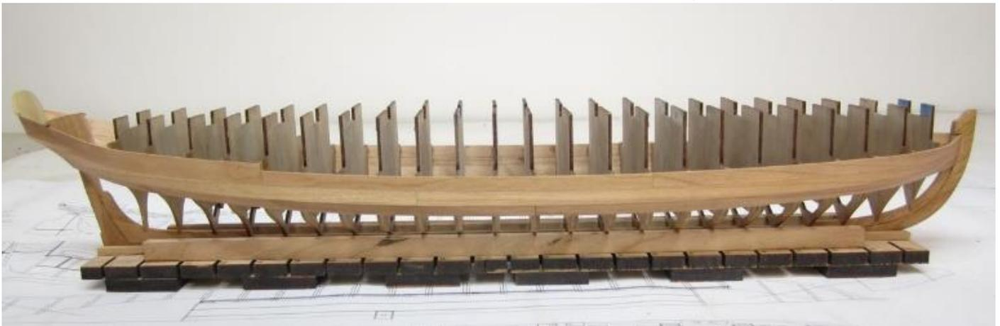
Do this slowly with a light touch and also use your other hand to hold the center steady as you file through the tabs. You can't see that in photo below because my other hand would have blocked the camera view of the tab being filed.
