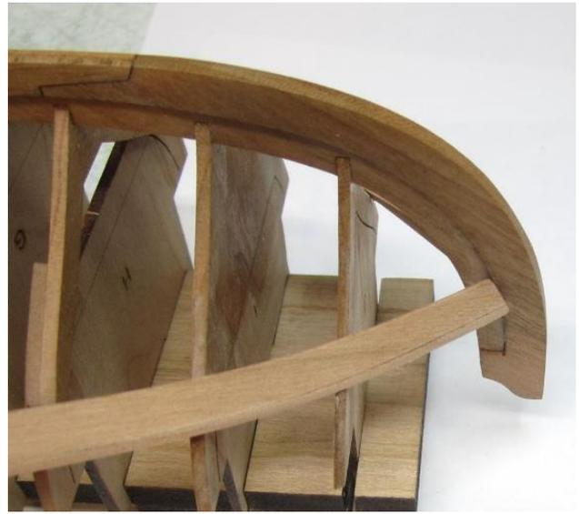
What you should see immediately is that the plank doesn't need much lateral bending at all. This isn't a very bluff or rounded hull. Just a slight lateral bend needs to be created.
