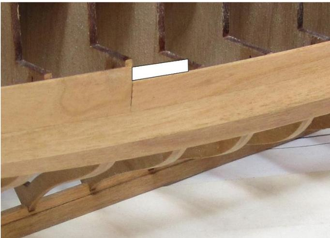
the frame centers to add this small piece of planking. Just remember to add it before you start gluing the cap rail in position. This is what I ended up doing.
