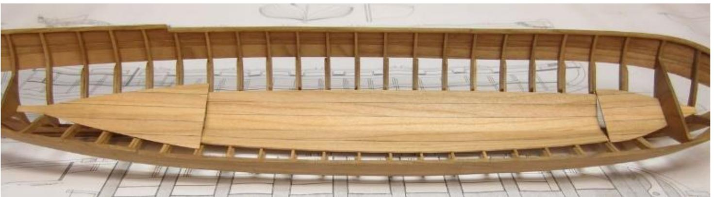
You can glue the aft platform into position but remember to use the depth gauge to find the proper depth for it inside your hull first. After you mark the sides of your frames and place the platform in position, it should fall at the same height as your tick marks.
