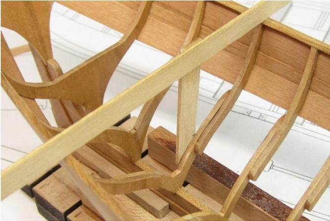
Then as shown above, rest the Depth gauge on top of the cap rail of your model along the frame you took your measurement from. Slide the tool left and right until the tick mark touches the top of the frame. Transfer this tick mark to your frame. This represents the proper depth for your aft platform at this frame. Repeat at each frame port and starboard and you will know just where your platform should be.
