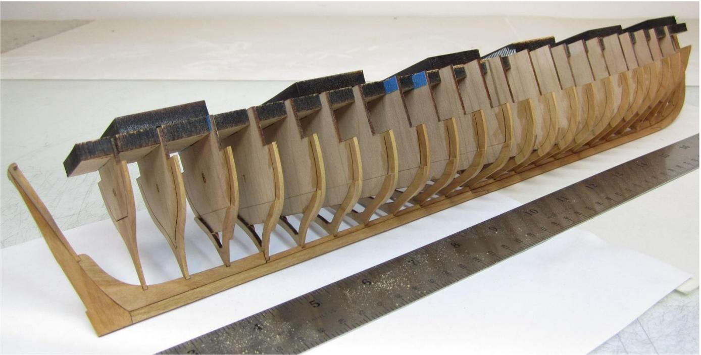
sanding as you move the sanding block back and forth. I personally prefer to use a sheet of sand paper for this and curl it up. I make sure that the fore and aft edges of the sandpaper are curled up so that it will not catch on any of the frames while moving it side to side.
