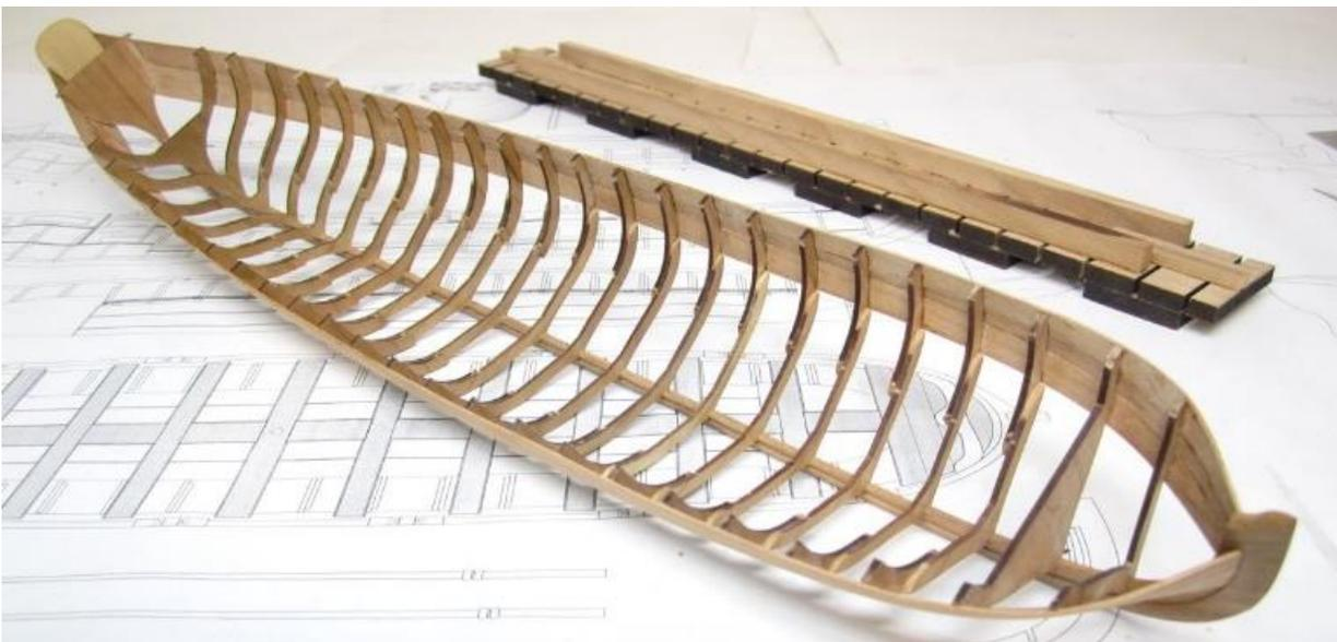
Then bend the frame center slowly and gently until the lower tabs break. REMEMBER, always bend in the direction towards the floors. This will minimize any tear-out to the floors and futtocks. See photos.
