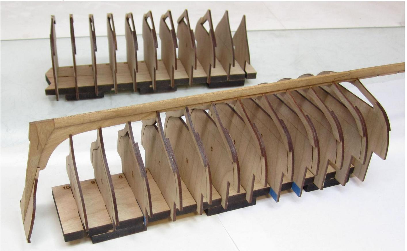
glue the keel in position permanently to this first half of the frames. Just like it is in that photo on the previous page.
