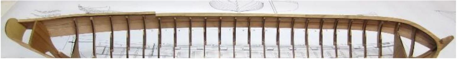
because you want to make sure the cap rail is glued down to the top edge of the planking as well as the top of each frame. It will give the entire hull much more strength that way.
