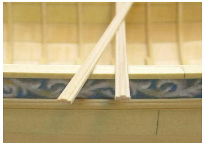
The last photo shows the profile I chose for the fancy molding below the frieze. This can be created in the usual way. The profile was filed into a thin piece of brass or you can use a razor blade. Then the scraper was lightly run over the boxwood strip until it created the profile you see in that photo. You can see a similar scraper below which was used on another project to create the fancy molding profile. This was done the same way.
