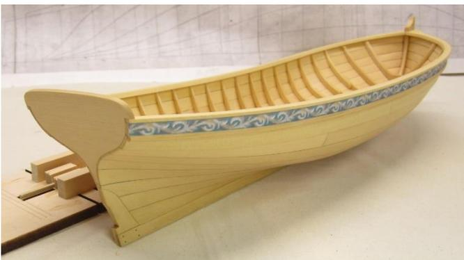
Use the bottom edge of the frieze to align the molding strip below it. The molding strip is  $1/8'' \times 3/64''$  and it is scraped to a simple profile. You were provided with boxwood strips for this in the kit.
