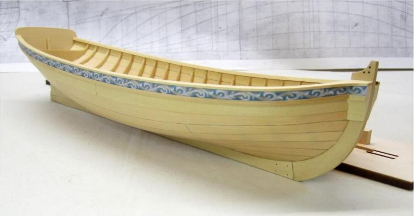
The friezes are provided already shaped like a pre-spiled plank. They should conform to the hull well enough. Try and hide the seam between the two halves mid ship as best you can and match the pattern like you would when you hang wallpaper. Then cut off any excess length at the stern flush with the transom. There is also a small length of frieze on your sheet that should be added to the bolsters at the bow. Cut off any excess flush with the front edge of the bolster.
