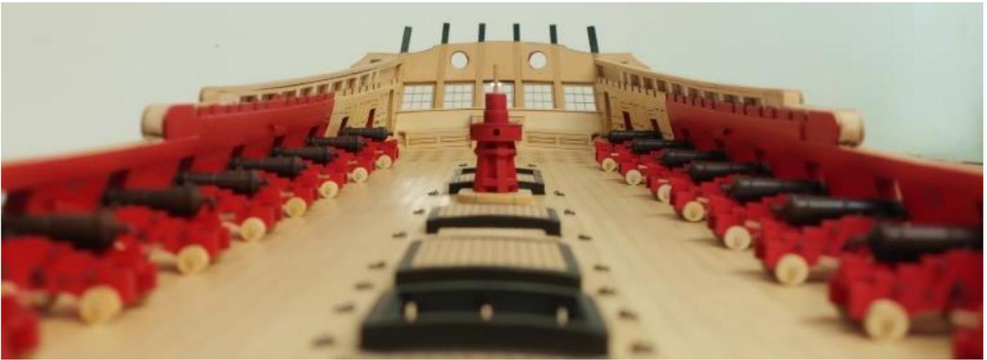
other fittings in the next chapter. But if you are going to rig them....this would be the time. Use 5/32" single blocks for the gun tackles using .018 tan rope. The breach rope should be roughly .045 to .050 in dia. As most contemporary models never showed the guns rigged unless the entire model was rigged, I will leave them unrigged as well.
