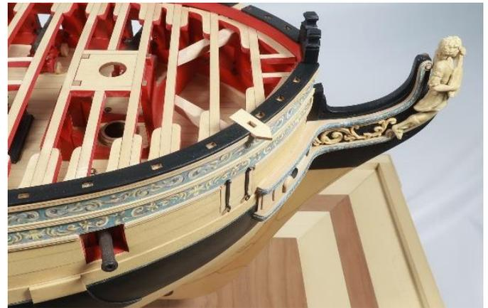
Then a laser cut spacer (looks like a small pointed arrow) the width of the catheads was used to help position the next longer piece on both sides. This is an important step. Its easier
