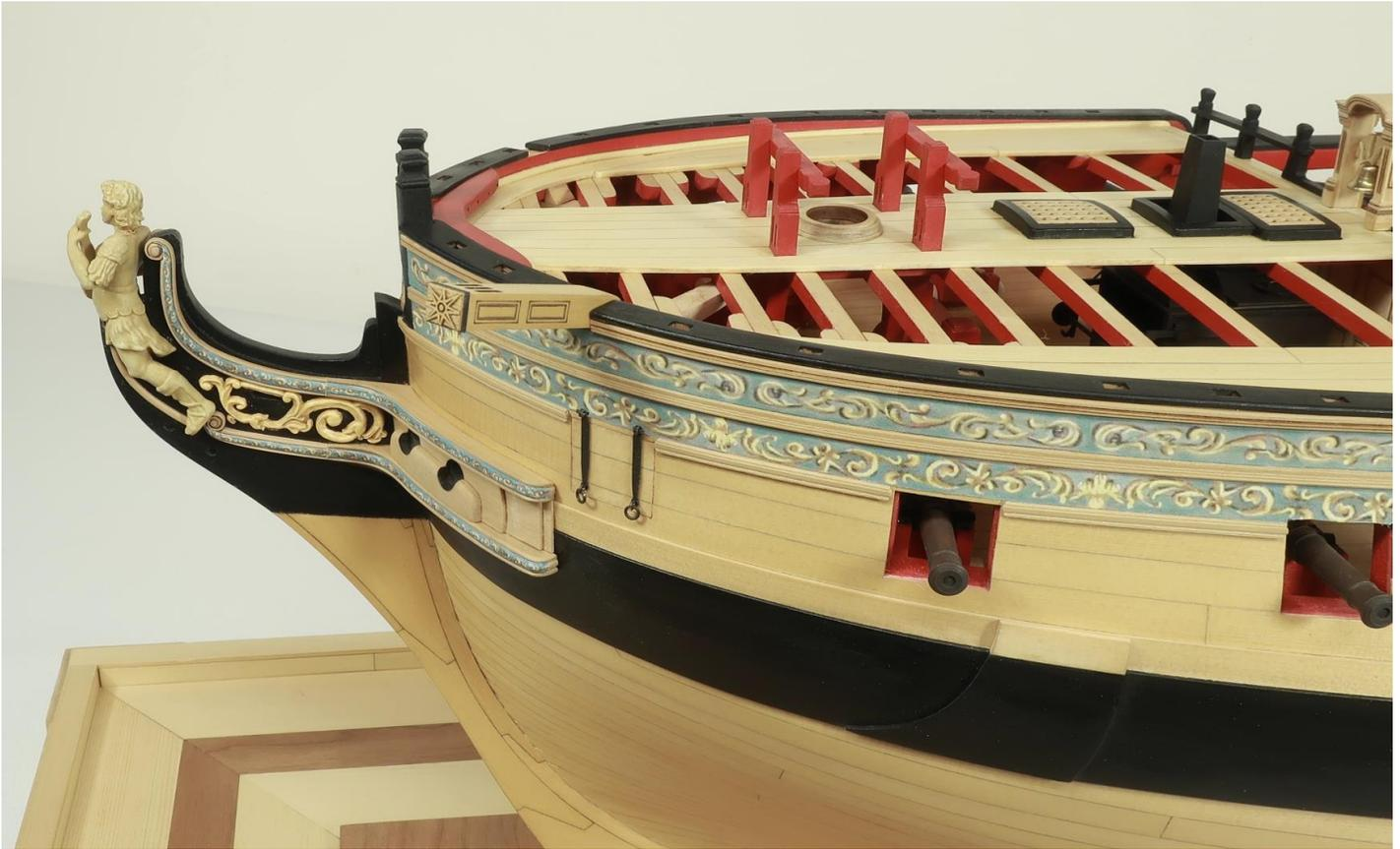
shown in models. The angle of the front of the cathead is important and before you glue the star onto it you should make sure its flat and shaped appropriately. Look at the laser cut sheet and I think you can better see the actual shape of the cathead on the side panels. I made sure I gave you guys an extra cathead just in case.
