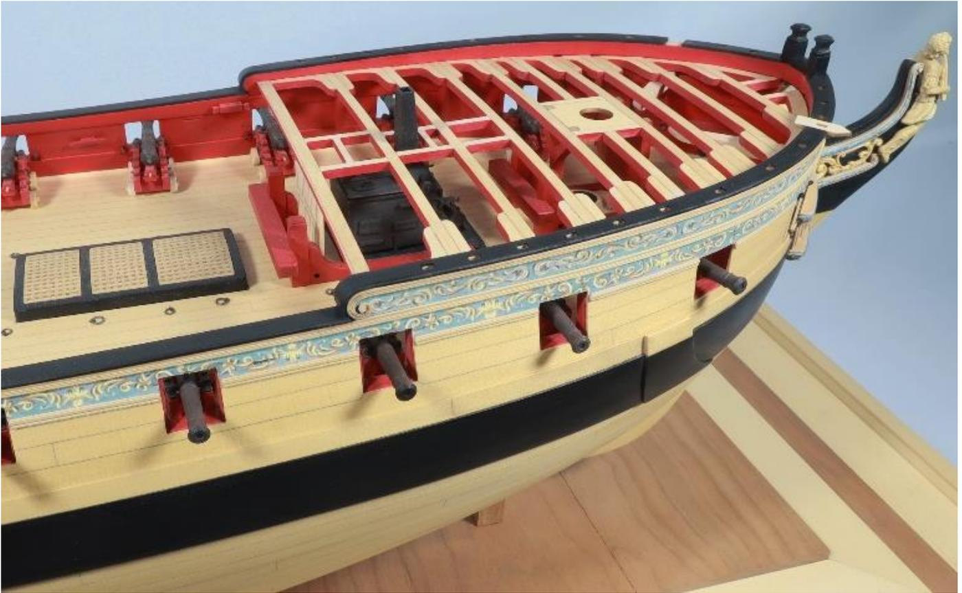
to widen the slot later and not so easy to make it smaller so be cautious here. Then the hance caps at the aft end of the fcastle were made as before. The two halves glued together so we have a nice wide piece. The hance caps were shaped and sanded for a snug fit. Then care
