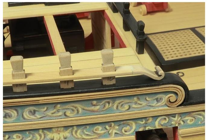
When dry, remove the entire rail from the model. Remove all the timberheads from the rail. I numbered the timberheads but that probably wasn't necessary. Then do your best to fill the seam between that fancy end piece
