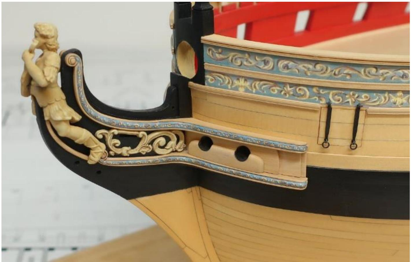
Here is a shot of the cheeks and hair brackets on the port side. Let me detail how they are made next. It's quite a long process even with most parts laser cut for you.
