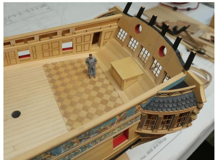
The benches are pretty simple as well. You just want to follow the curve of your transom. This might be different slightly from model to model. First, you add one of the bench sides to the side of the rudder trunk. See below. Note how the top aft point of the side is even with the break along the inboard counter.
