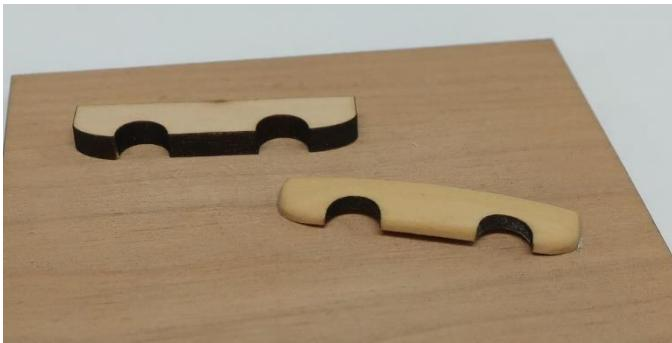
Then shape the forward side keeping it a consistent thickness. To finish it up round off the top edge as shown. **IMPORTANT NOTE:** Do not glue this in position. Just make sure it fits and looks good sitting on the cheeks. You don't want this glued on when you drill out the hawse holes. We will be doing that next. They would certainly get damaged.
