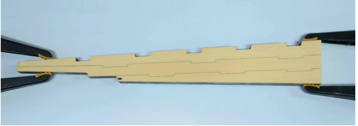
*Assembling the three laser cut rudder sections...*
