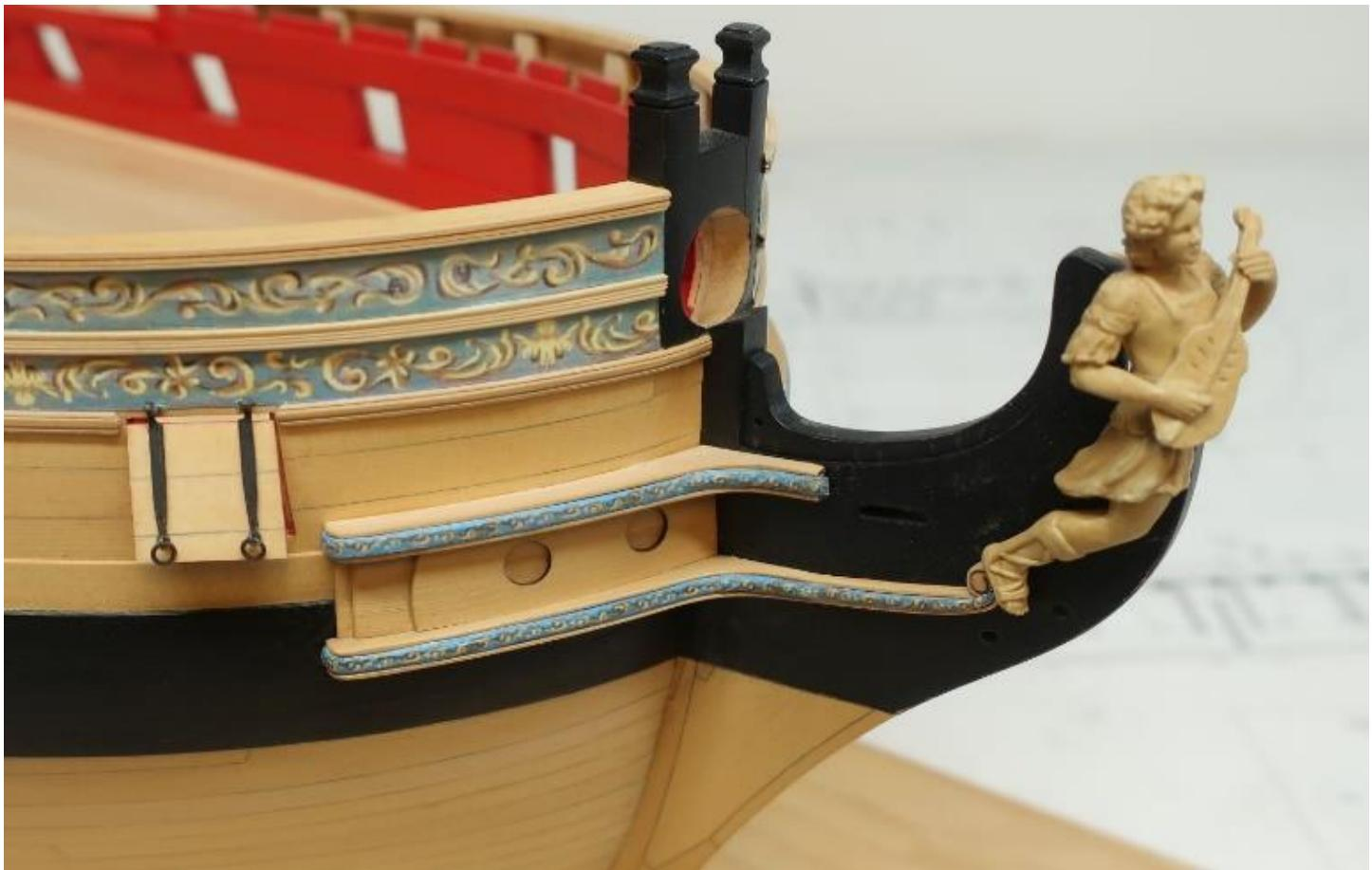
Next is the upper cheek...You should have beveled this like the lower cheek. This one should go easier. Note how it wraps onto the stem. It doesn't extend above the top of the stem. This upper cheek is also shorter on the hull as you can see. You can also use the trailboard carving to help you position this. Make sure you have enough room for the carving.
