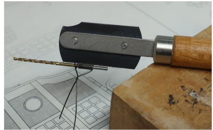
hinge straps. Note the left and right hinge straps on the lid. This is done so the little "L's" are both on the inside. Then your lid will never fall off after you glue it on the hull.
