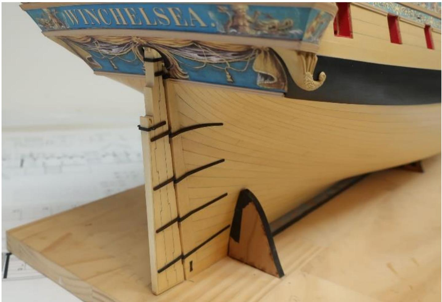
I also added the horse shoe plate at the bow along the gripe. This is also laser cut for
