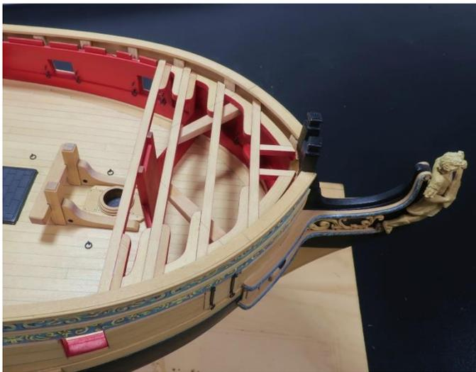
Above is a photo showing the cat tails glued to the underside of the deck beams. Note the pencil reference marks on the bulwarks from the templates. These were very useful. Also note the very light reference marks I drew on the top of the deck beams to help me position the cat tails before the glue dried. I used PVA glue so I could manipulate and move the cat tails in the correct position matching my reference marks.
