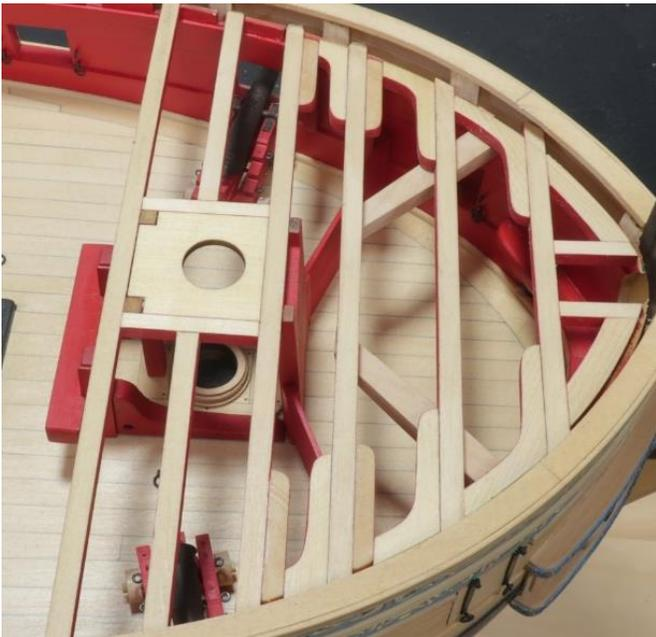
The photo above shows the fore mast partner glued in position. This was done first. Note how the partners are notched around the "y" bitts. In addition, the mast hole is actually aligned with the mast coat below it. This doesn't matter so much since we won't be rigging the model or adding stump masts.
