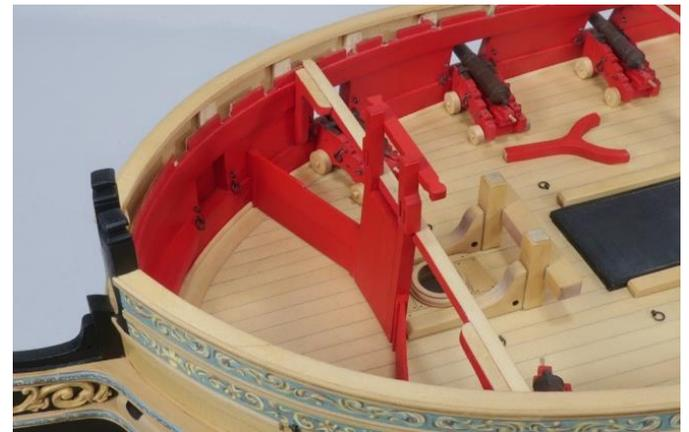
beam from the stem. That should be installed first so you can sit the bowsprit step against it.
