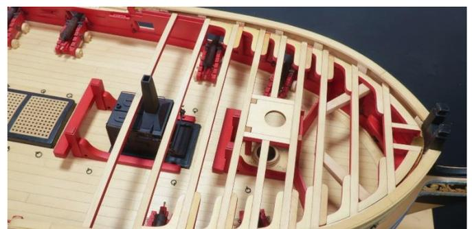
In the photo above you can see I added a few more beams and the knees required. But then I had to glue that stove and drip pan in position permanently before I could do any more of them. I kept using the template to check positions. The aft riding bitts were glued on permanently as well. The stack for the stove is only lightly glued on the stove. I needed to
