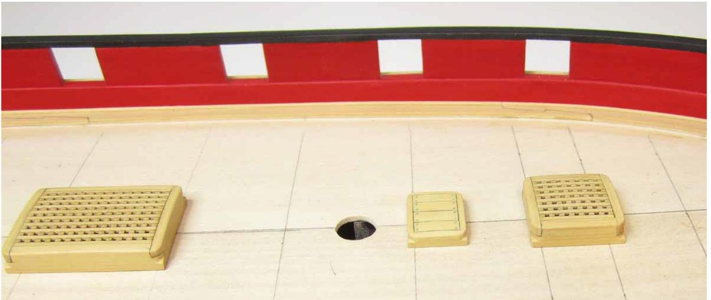
Repeat this process to make the final grating and coaming but be sure to measure its height from the plans. In addition, you can make the small coaming for the galley stack. There is no grating but instead it is covered with planks. There measurements can be taken from the plans. It is different in that the coaming is only 1/6" thick and it is not as tall as the other two.
