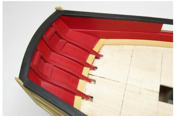
With these completed, I started fabricating the margin plank for each side of the model. Each side will be made up of three sections joined with scarp joints. Examine the plans for their locations. The photo at the top of the page shows the three segments cut in advance and test fit on the model. The edges for the scarp joints were darkened with pencil before gluing them onto the model permanently.
