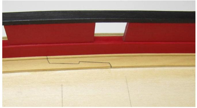
Note the seam between the two lengths of waterway conform to the seam of the scarp joint in the above photo.
