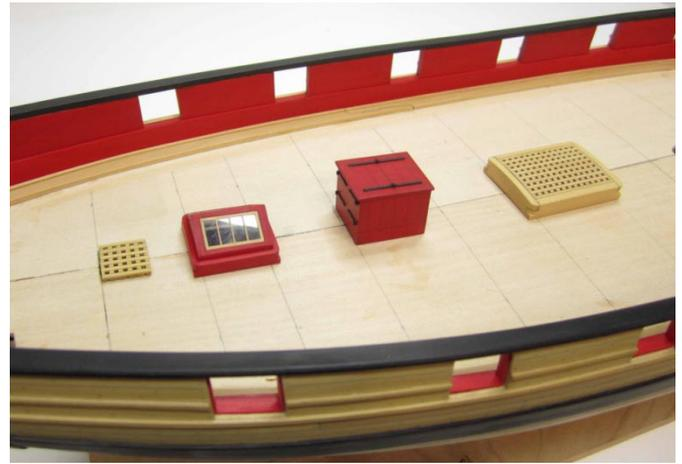
All of the six deck structures and fittings were finally glued onto the deck. Careful attention was paid to ensure they were positioned correctly down the center line of the deck.
