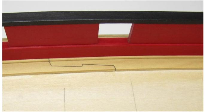
Note the seam between the two lengths of waterway conform to the seam of the scarf joint in the above photo.
