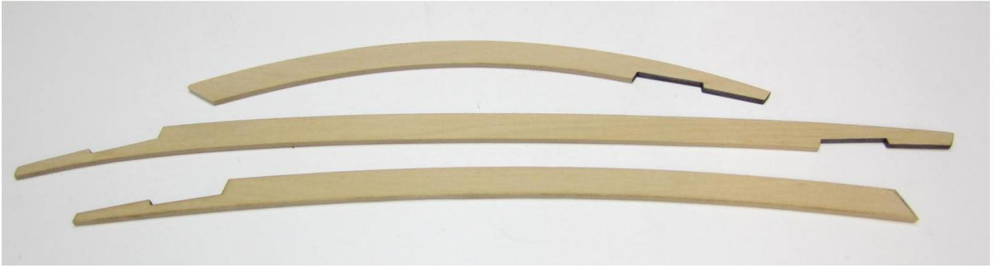
Three sections of margin plank have been cut for the port side.
