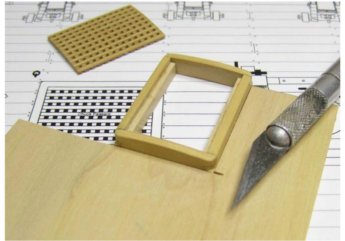
The photo above shows the corners being rounded off. The rounded corners are only above the deck planking. To make this easier, I created a small "right-angle" jig the same thickness as my planking. The deck planking will be 3/64" thick. Hold the corner in the jig and use a sharp blade to carefully slice the corner down to the top of the jig. Then round it off with a file or sanding stick.
