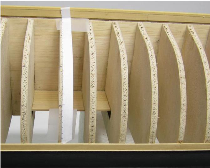
I find using a planking fan another good technique for quickly dividing a tick strip equally into segments of any width. I have provided one for you on the next page. Just lay the strip on top of the planking fan which has equally spaced radiating lines. Moving the strip evenly up and down will give you perfectly spaced segments. I have already marked a center line where the segments are  $\frac{3}{16}$ " wide. Just lay your tick strip across the
