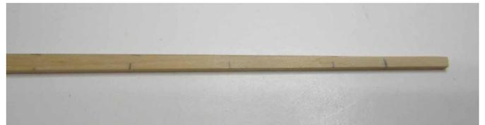
6. Now it is time to bend the plank edgewise. How do you determine the curve you will need. I usually hold the plank in position without bending it. I allow it to run naturally against the planks already on the hull more or less. This doesn't have to be exact. You want to reveal the gap between this plank and the one already on the hull. See below. Mark the widest point on the plank, or the apex of the curve.
