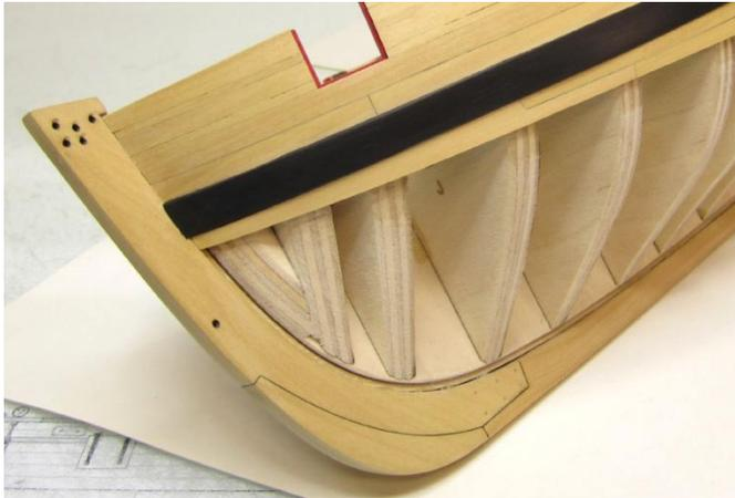
For now, I just added the first strake under the wales. It terminates at bulkhead "J" as shown on the plans. Forward of this strake will be the drop plank. This strip was added below the wales and remained a constant 3/16" wide until it reached bulkhead "b". From here until it terminated at bulkhead "J" is gradually tapered to 5/64" wide. You can actually follow the plan very closely here.
