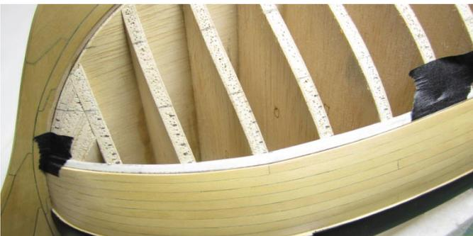
1. Don't forget to mark all the locations for your butt ends on each bulkhead. It will be easier to follow and create a consistent planking shift pattern this way.
