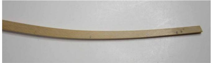
8. Bending the plank edgewise is only half the fun. In order to place the plank on the model without forcing it, you will need to bend it again to fit the curve of the bow. This is easy. Just clamp the end to the table and gently bend it while applying heat with the blow dryer. Note how the finished plank is curved in both directions now and will fit nicely in position against the last strake you put on the model. No forcing at all!!!
