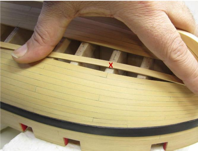
7. Using this reference point I can clamp the strip into position with an estimation of the curve needed. I always “over bend” the plank to compensate for any spring back after its bent. In this case I had to mark the apex on the other side of the plank because it needed to be flipped over to bend it in the correct direction. This will make sense once you give it a try. On the other side of the hull it isn’t necessary. I am bending it clamped to the edge of a piece of wood.
