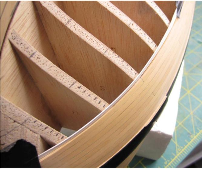
When the curved template is used, the plank fits flat against all bulkhead edges and no forcing is needed. See below. The big question is how to determine what this curve is. There are any ways. But here is how I did it for Cheerful.
