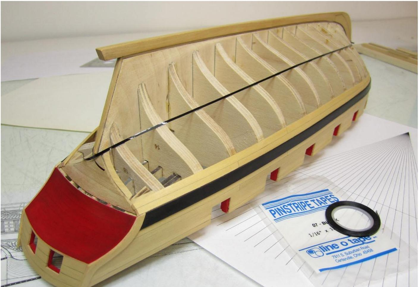
The pinstripe tape is self adhesive so once you have the locations at the bow and stern, you should adjust it at every bulkhead edge until you have a smooth run. Take your time examining the run of your tape as it will become the run of your planks. Make tiny adjustments until its smooth and true when viewing it from every angle. I do this on both sides of the hull to ensure it is the same.
