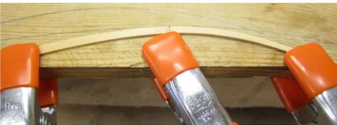
The center clamp is just used as the pivot point against the apex of the bend. Its not actually clamping down on the wood. It does however stop the plank from lifting off the wood while bending.
