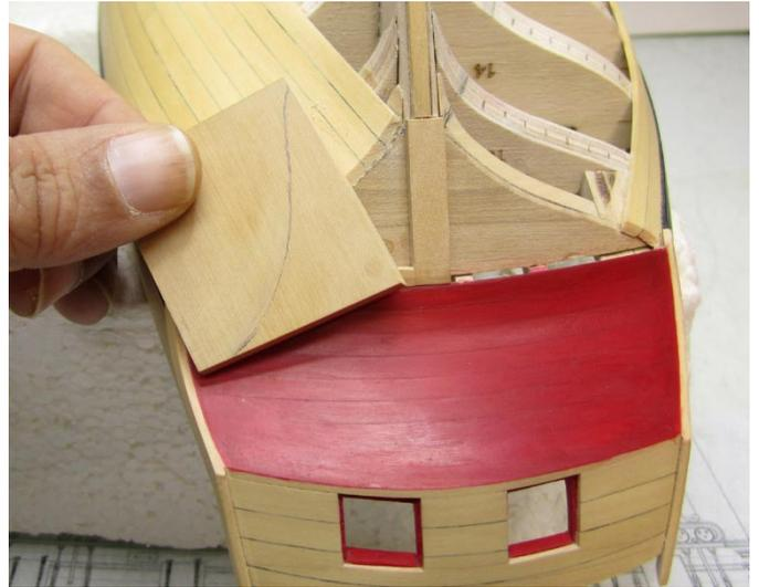
Cut it out with your scroll saw. You can make it slightly over-sized at this point. Here is the tricky part. Go ahead and glue this to the square tuck...but not permanently. You need to be able to remove it after you fair it. I did this by adding just one or two drops of CA to the square tuck. It was just enough to hold it securely but still allow me to pry it off after I was done.
