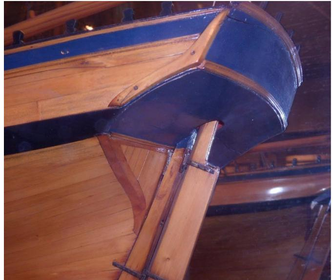
The rabbet strip should be flush with the outside of this strip so the stern post will sit flush against both later in the project. You can see this strip in the image below.
