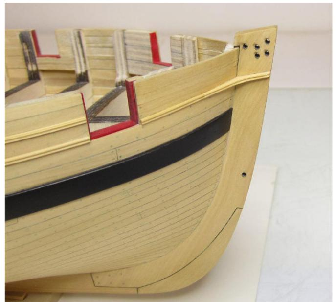
Its best to fit the small "ear" that crosses over onto the stem first. Then add the small length of molding behind it. The tricky part will be matching the beaded profile along the edge of the ear. This was scraped into the edge of the "ear" using the same scraper.
