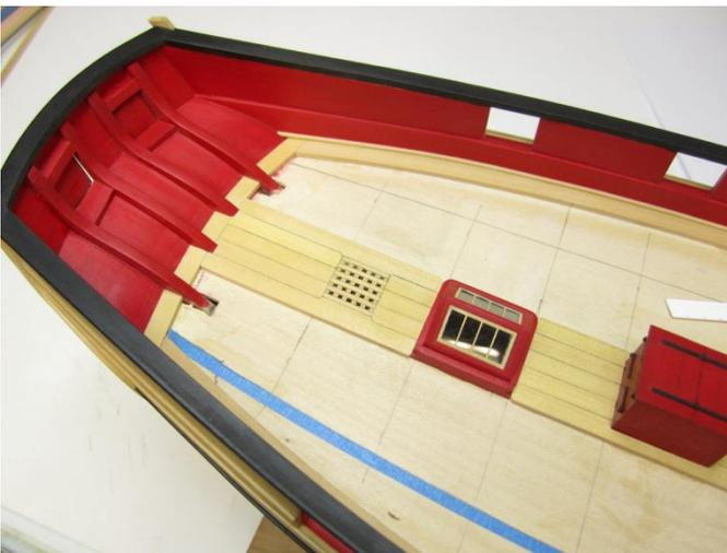
**Only the three outer planks in the outer belt will have hooked scarphs on the plank ends.**
