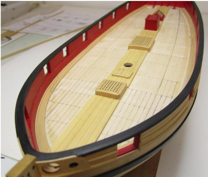
The photo above shows how I actually drew the planks onto the false deck. I did this at the stern and at the bow. It allowed me to see the shape of the scarphed planks. They are actually called hook scarphs.
