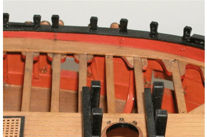
Note how the scarphed planks sit against the waterway rather than being cut into it as shown on the plans. The same will be done at the stern on the *Cheerful* model. To do this, we must line-off the deck in much the same way that we did for the external hull planking.
