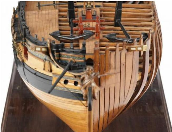
The photo above of the frigate Winchelsea 1763 shows a contemporary example of this curved decked planking at the bow. Another good example can be seen on the contemporary model of the frigate Minerva in the Rogers collection. You can see how the deck planks at the bow are curved and
