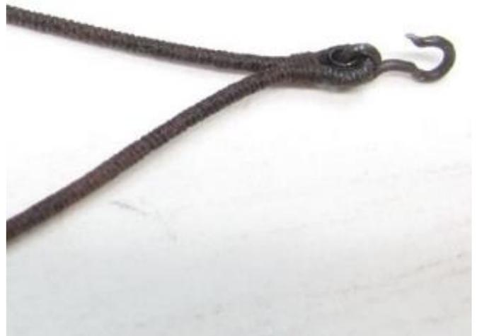
A served rope basically has a thinner line wrapped around it as shown above. It can be needed for a ropes entire length. The serving machine allows you to wrap a standard rope with a thin thread for an unlimited length. See below for a photo showing a served line ...bottom...in comparison to a non-served length of rope.
