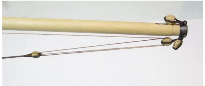
extremely important when I turn in the deadeyes for the shrouds and set up the backstays. Once the backstays are rigged it has a tendency to make the aft shrouds go a bit slack....being able to re-tension is a huge plus so none of the lines will be made permanent until much later, if at all. The rigging is not pulled to tight at this point. Just enough tension so it doesn't go slack. I see so many models with the rigging so tight it causes big issues.
