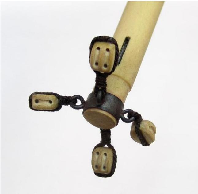
This end is hooked to the eyebolt at the bow. They are hooked to the eyebolts on the sides of the bowsprit that have the 3/16" single blocks on them. These cutters had many lines that sometimes utilized the same belaying point or eyebolt etc. Take a look at this photo below of a contemporary model of a cutter from the same time period.
