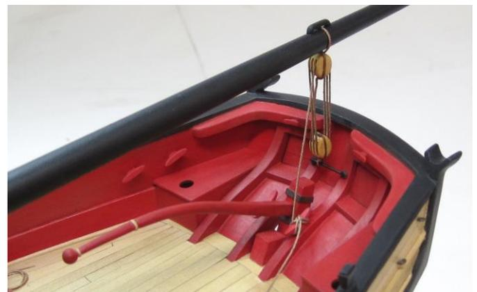
Run that line through the triple blocks. Take the loose end and secure it to the cleat on the stern frame as shown. But no glue as before. Tension it so the boom is pulled down tight but...not too tight. You don’t want to pull the mast back or bend the boom etc. Just make it snug. After a little time the rigging will relax and you will have to make it tighter.
