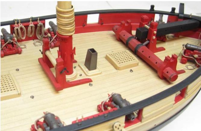
Then the masthead area from the bottom of the cheeks upwards was painted black. That was done after adding the mast bands and eyebolts. These will be used for the boom and gaff rigging later. I used painters tape for the bands. The tape was painted black and then cut into thin strips the same
