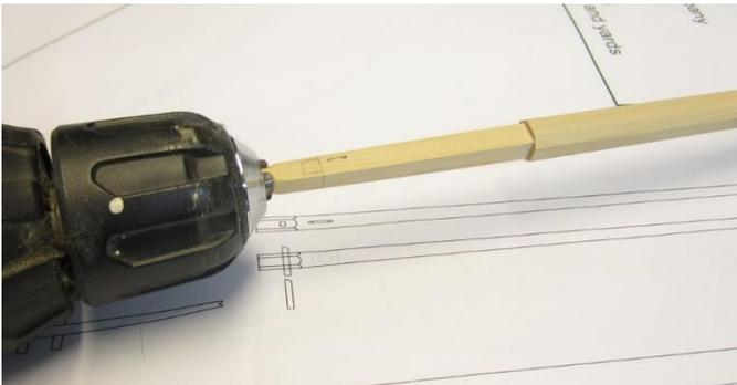
It was chocked and rounded off with some sandpaper. I also carefully created the taper to the rounded portion while sanding it. The mast has a slight taper to a smaller diameter as you get closer to the squared off section at the top of the mast.
