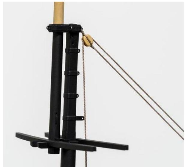
block you seized to the tip of the boom. Then it is brought back up to the block on the cap. The long running end is now ready for you to create the topping lift tackle secured on deck. The boom should still be just resting atop the transom at this point.
