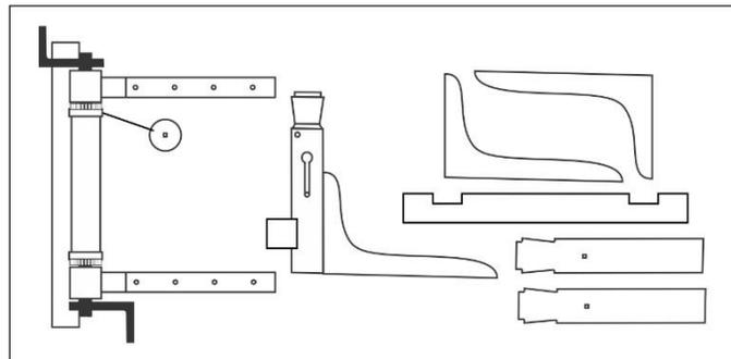
The only remaining parts of the winch were its handles. There are many ways to make these. I used a small thin piece of boxwood with a hole drilled through its end. Then a piece of 24 gauge wire was inserted into this hole to simulate the crank handle. To finish it off, a small (very tiny) length of micro tubing was glued onto the end of the crank handle wire. This gave it more detail and finished it off nicely.
