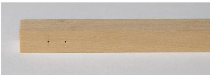
Step two – prepare the outboard end of the bowsprit for rounding. To do this, use the 7-10-7 ratio just like we did when making the octagon pump tubes. The outboard end of the bowsprit will be planed, or filed to an octagon before you can make it round. So mark each side of the stick with lines using the 7-10-7 ratios. See below.
