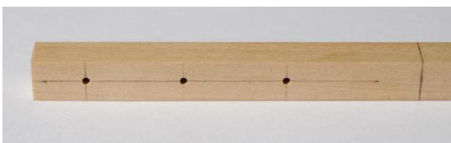
There is also a sheave on the outboard end. The holes for this sheave is simulated also. It is also drilled while the stick is square. Make sure you drill through the right side of the stick. Study the plans carefully.
