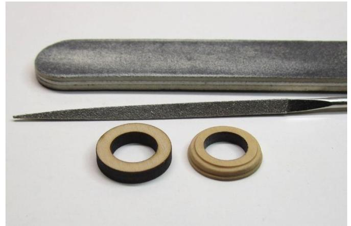
Many contemporary models have stylized mast coats with a fancy profile. A small washer of 1/8" thick boxwood was made. Now if you are fortunate enough to have a lathe or even a vertical milling machine, there would be countless ways that you could make the mast coat. But if by chance you do not, the mast coat can be shaped by hand by careful use of needle files, emery boards and sanding sticks. This is the method I chose to use and the photo above shows the results.
