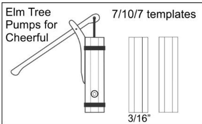
1. Transfer the 7/10/7 template lines to each side of the 3/16" square pump tubes. Carefully file the tube to an Octagon using the lines as a guide. Drill and bore out the top of the tube to a depth of about 3/8". Carefully use a bit that will leave the pump tube walls not too heavy.
