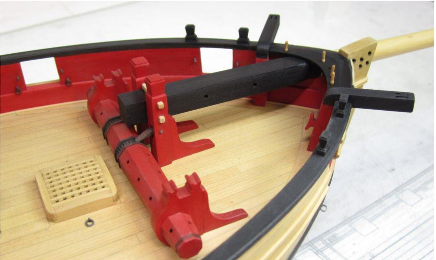
Note that in the photo above, the bottom cross beam of the bowsprit step looks like it goes through the bowsprit. But it does not. It's only simulated because it was easier to slip it over the top of the bowsprit.
