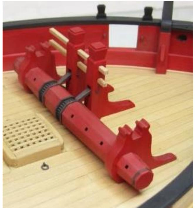
above. The two boxwood strips left a bit long for the time being. They will be cut to their proper length after the bowsprit is made. For now however, just set the bowsprit step aside and begin making the bowsprit.
