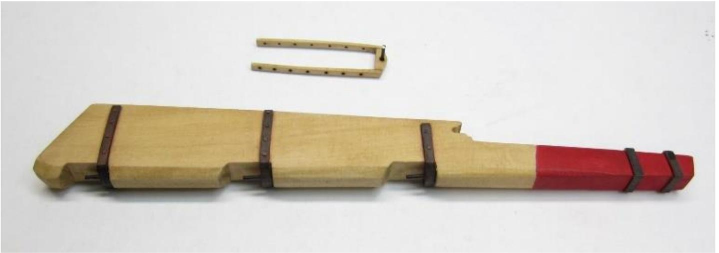
edges. The rudder is tapered as it works its way aft. The profile for this tapering is shown on the plans. The taper also exists as the rudder proceeds down to the bottom edge. The photos also show the shape.
