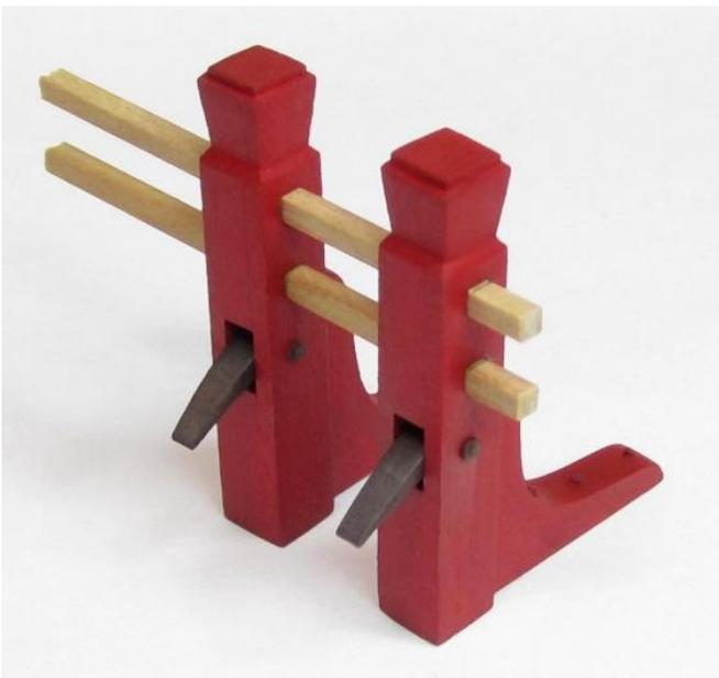
The pawls were painted black and weathered to look like metal. Placing them in the mortice of each upright, they were held in position with a small length of black wire fed through the holes laser cut in each piece. This actually makes the pawls movable so you can adjust them as you position the bowsprit step alongside the windlass.
