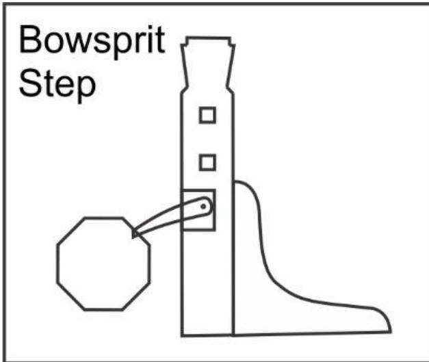
Assemble the three layers for the uprights. Then use a needle file and sharp chisels to finish shaping the top of both of them. They will look like the timberheads along the cap rail and the top of the winch uprights when you are done.
