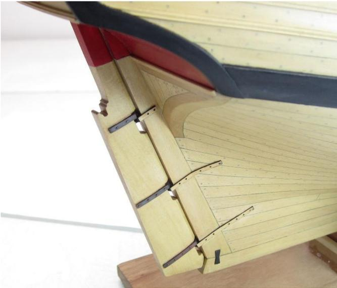
The rudder was hung as a test so I could mark the area of the rudder head that was to be painted red. I also used some weathering powder on those pintles and gudgeons so they would more realistically look like simulated metal. The same thin material was used to simulate the two metal band around the rudder head.
