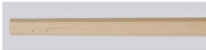
Step three – I then chocked the square end in my power drill and proceeded to make the octagon section round. Running sandpaper up and down along its length as the bowsprit turned at high speed. At the same time I carefully tapered the outboard end smaller to match the shape shown
