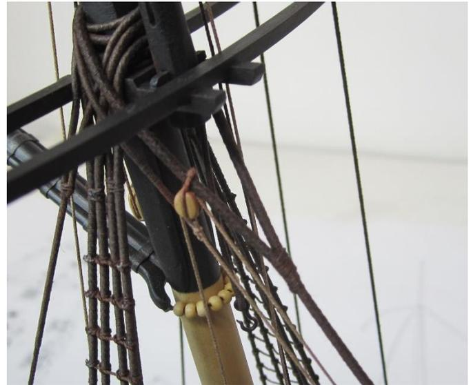
belayed to a cleat around the base of the lower mast.
