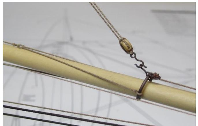
The loose end was brought inboard to the bowsprit step upright on the port side.
