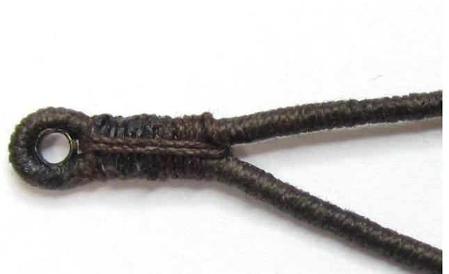
the center of the seizing as shown above. Twice around is just fine. Glue it in place and this half of the sling is completed.
