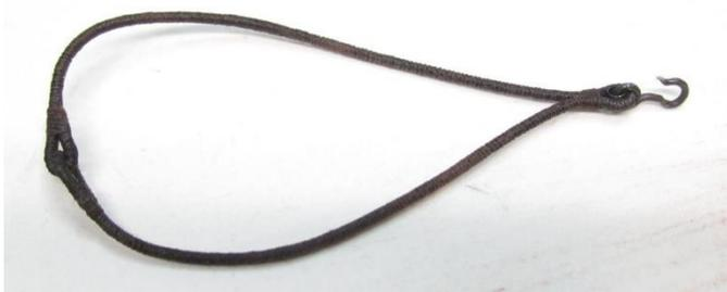
contemporary models the closed eyes are not equal lengths away from the hook. The eye is offset to one side so it ends up on the port side of the shroud gang. To simplify this I just made equal lengths and tried to make sure the hook ended up hanging where it should be. This is a tricky item to make.
