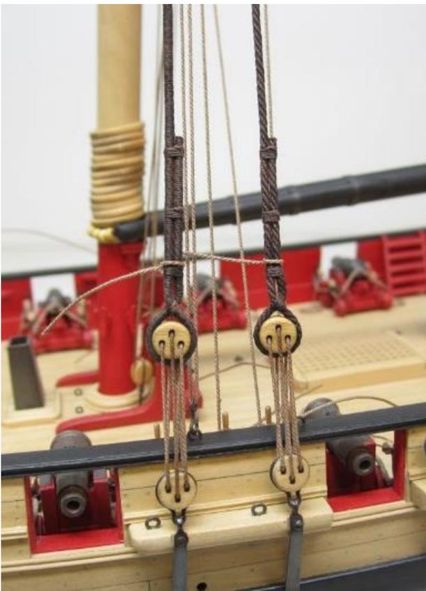
The next pair was completed on the starboard side. Then the process was repeated. Here is a look at the four shrouds and deadeyes set up on the port side.
