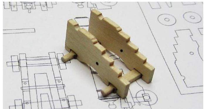
**STEP THREE** – Add the laser cut transom on top of the front axle. See the plan for details on its angle. Another small strip is placed in top of the rear axle. To finish off this step, a length of 22 gauge wire is pushed through the holes on each bracket. The wire should be cut so it stands proud of the surface of each bracket. Just by a little bit to resemble a bolt head!!! Larger wheels (trucks) go on the front of the carriage. See the photos.
