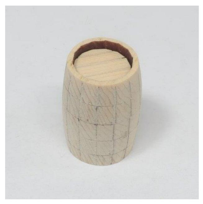
So once the top and bottom are glued into the ends....sand the ends shorter until you have just a small lip like the next photo.
