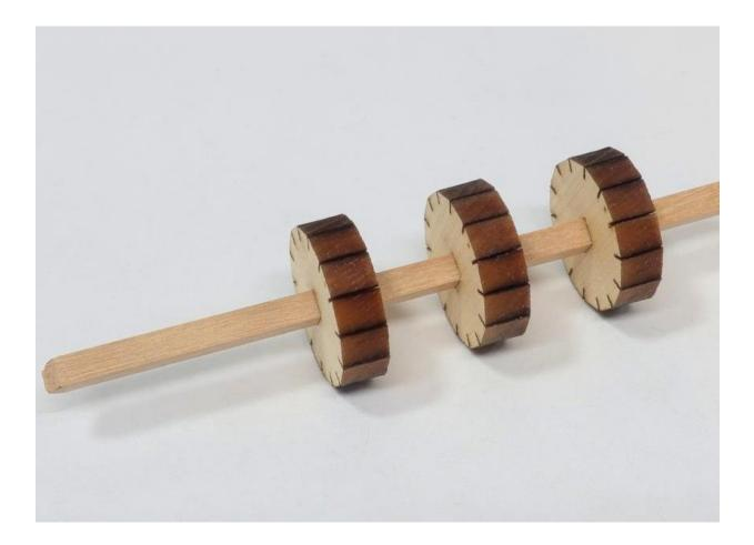
Pull the three or four center layers off the stick and glue the "ring" layers on each end. Once again, look for the alignment dot and have them face the same way and be lined up.
