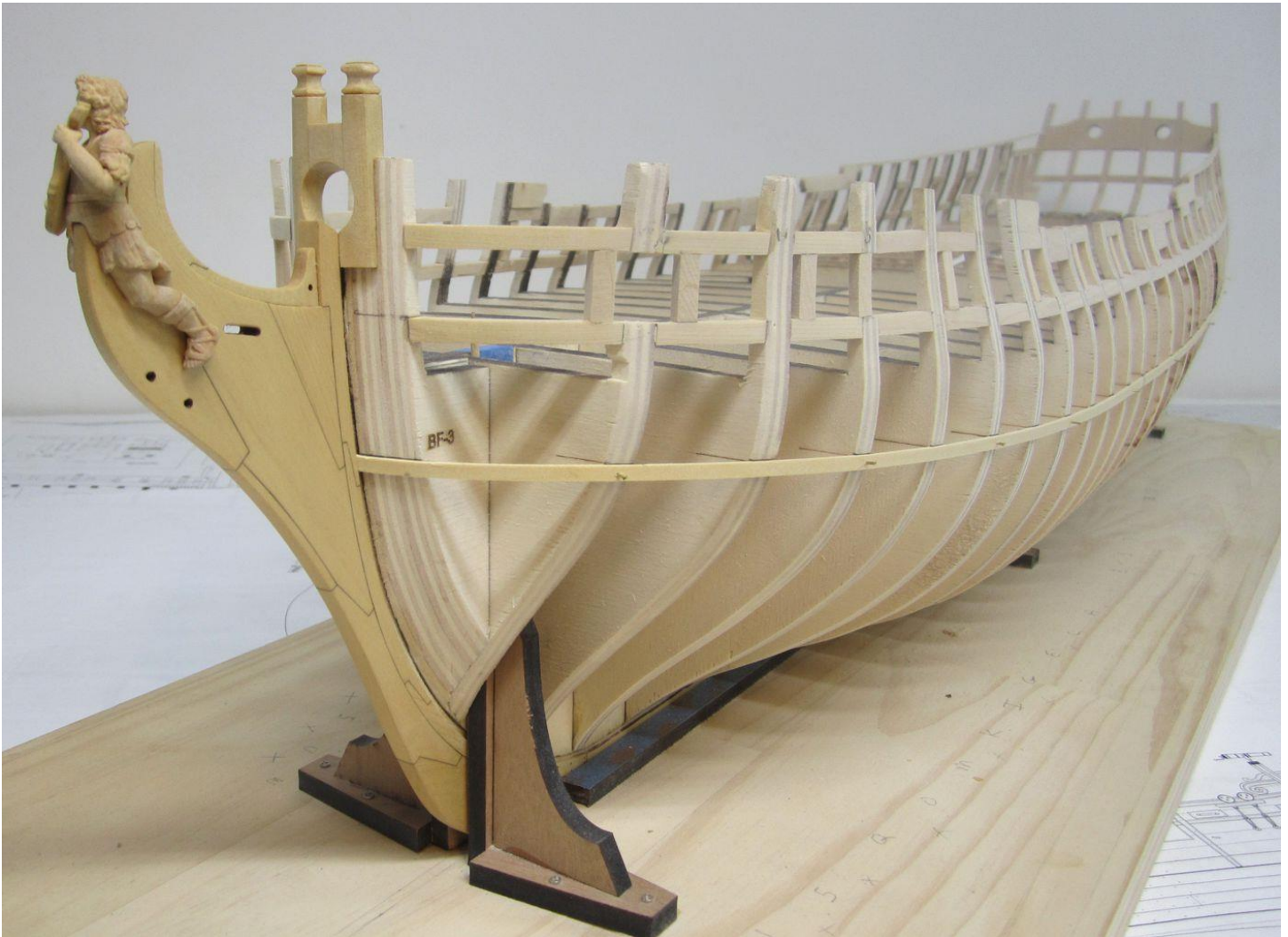
View of the model with a batten in position that locates the bottom edge of the wales.
