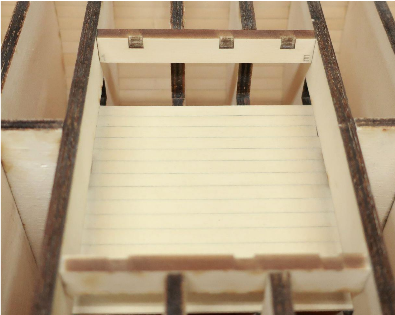
View of the first two parts used to frame the hatches
